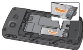
4. To insert the battery, align the golden contacts of the battery with the corresponding connectors on the battery compartment. Press down on the opposite end of the battery until it snaps into place.
